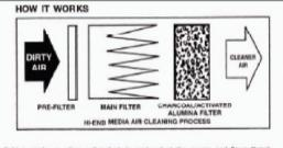
Solder, smoke or other poliuted air is captured at the source and flows throigh the arm or arms, through the foam prefilter. This prefilter effectively removes the large particles. Next the smaller particles of poliuted air are captured by the Hepa-type filter and flurnes are absorbed by the charcoa/activated alumina filter. The air that is discharged is then poliution-free.
